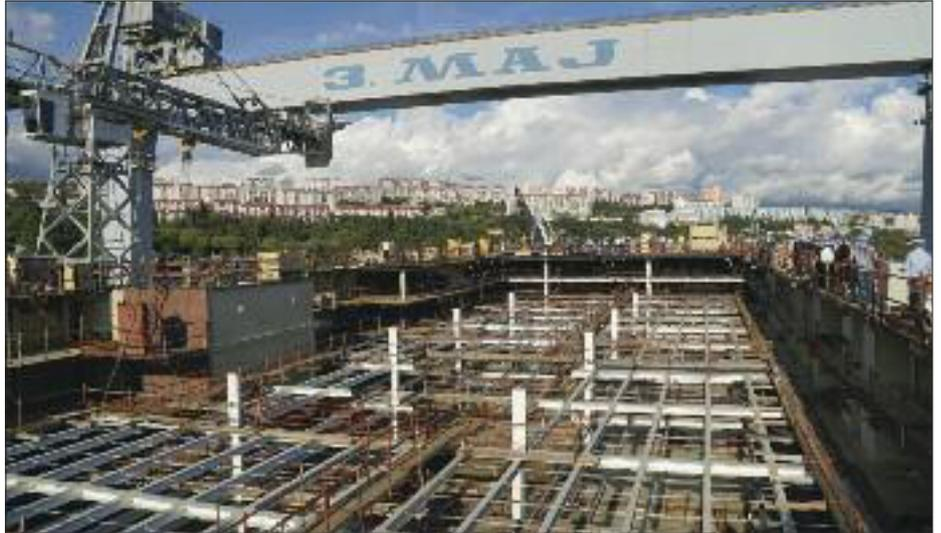
'Siem Cicero', the first car carrier to use composite materials in its cargo deck structure, being built at 3 Maj
