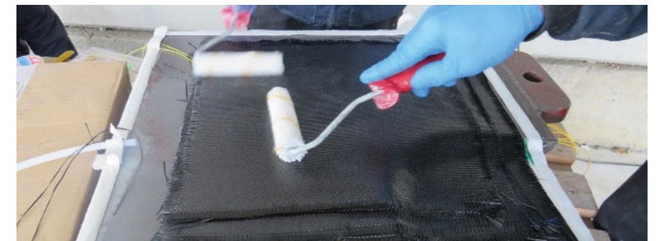
Composite Patch design by FEA analyses (left). Patch Manufacturing process (HLU+VB) with optical fibers embedded among layer (right)
