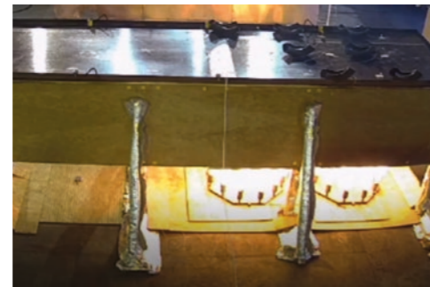
Cardeck panel for Flow Ship Design, full scale fire test of cardeck panel at RISE
