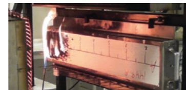
Spread of flame test at RISE.
