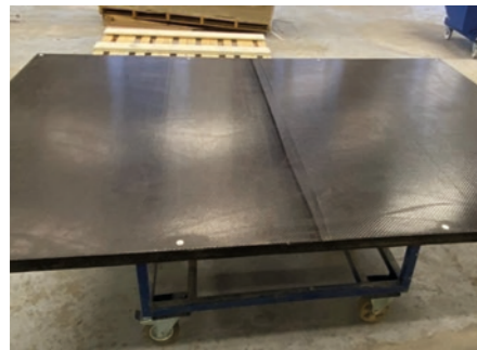
One panel as delivered and one with PVC-foil at Meyer Werft
