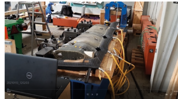
Measured deflections on composite rudder flap under load.
