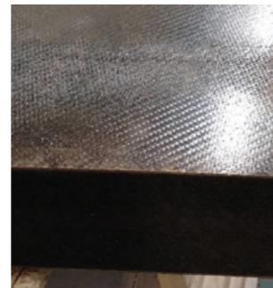
Acoustic panel from PFA/glass prepreg and FoamGlas core
