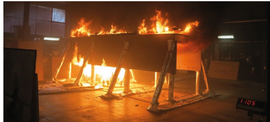
Large scale fire testing of a ro-ro deck structure at RISE
