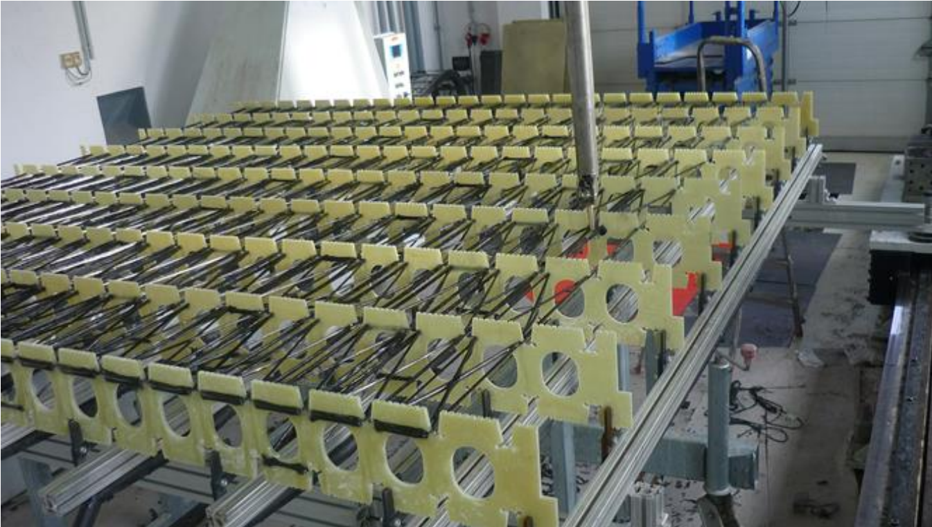
Laying of strands to build a plate
